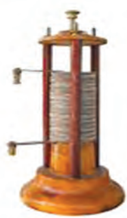
Volta's simple electric cell
